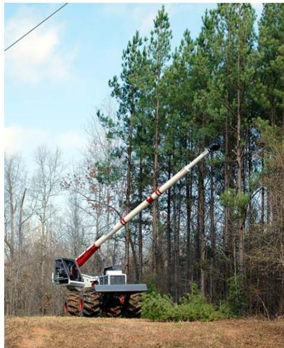
Figure 2 - Mechanical Side-Trimmer
